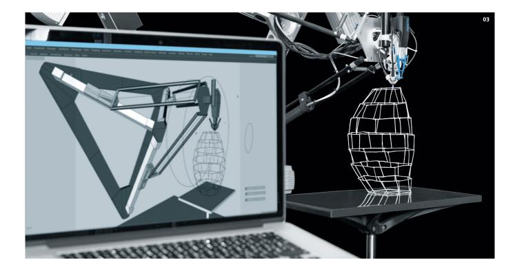
Particularly in sectors like the packaging industry or medical technology, a host of new possibilities are opened up by this technology. By integrating the spinneret into the tripod, the developers are also testing how existing standard components can be enhanced for digital fabrication, and hence the production tasks of the future.
