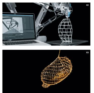
The tripod receives the necessary positional data and control signals directly from an animation software program that is normally used to create virtual 3D models, computer graphics and simulations.
