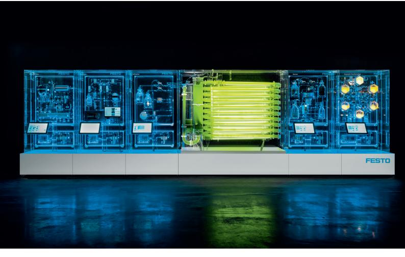
01: BionicCellFactory: Holistic bioprocess in five modules 02: **PhotoBionicCell:** Our first bioreactor with a capacity of 10 litres for the automated cultivation of algae.
