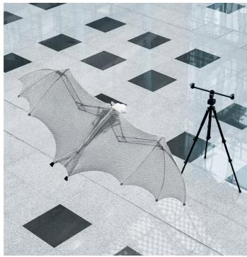
Besides the ingenious kinematics, the artificial flying fox also owes its agility to its lightweight design and clever use of materials; its body is made of foam, whilst the skeleton consists of milled carbon rods and 3D-printed parts.
