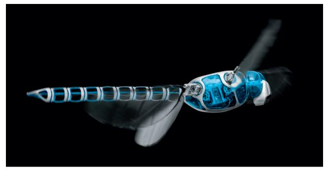
Intelligently combined: the interaction of open- and closed-loop control systems enables the flying object to take nearly any orientation in space
