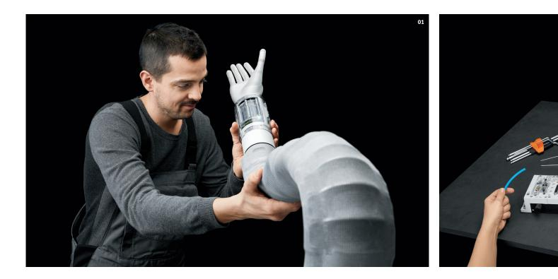
In order to keep the effort of tubing the BionicSoftHand as low as possible, the developers have specially designed a small, digitally controlled valve terminal, which is mounted directly on the hand. This means that the tubes for controlling the gripper fingers do not have to be pulled through the entire robot arm. Thus, the BionicSoftHand can be quickly and easily connected and operated with only one tube each for supply air and exhaust air.
