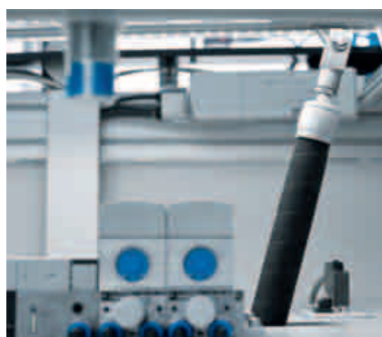
Tilting the field with compressed air: the DMS-20 pneumatic muscles
