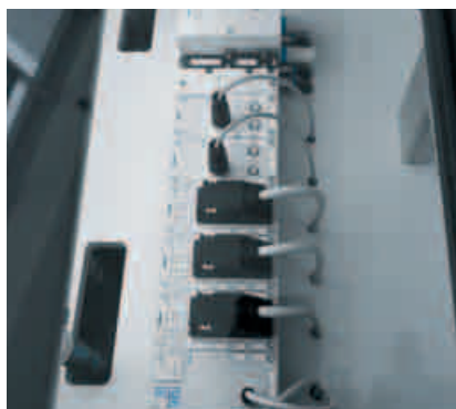
Precise control of all components: the CPX /MPA valve terminal
