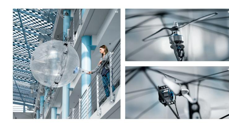
The propellers on the FreeMotionHandling are no longer located directly on the ball, unlike the eMotionSpheres. Just like the entire onboard electronics, the eight adaptive drives are fitted on the ultralight flying ring, which could thus also be used without the helium ball.
