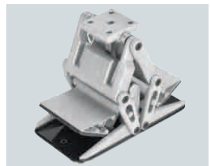
Gentle detachment of the film from the gripped object by deformation of the structure with Fin Ray Effect®
