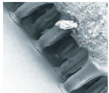
The gripper under the microscope: the nanostructure of the foil magnified 400 times
