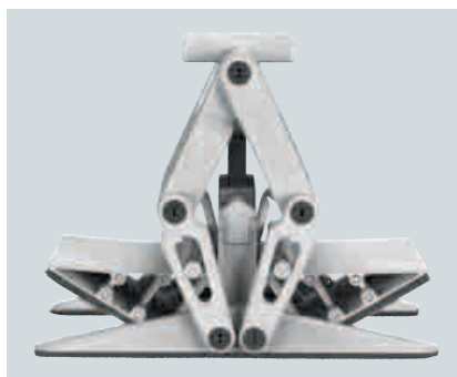
Push-push mechanism: the structure is activated without additional actuators or control components
