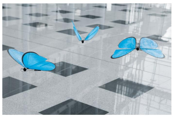
The on-board electronics allow the two pairs of wings to be precisely activated and contain their own inertial sensor system to control the flying behaviour. Using the two servomotors, the beat amplitude, beat speed and the respective turning points can be freely and individually selected. In this way, the eMotionButterflies are fully manoeuvrable, very agile and come extremely close to their biological role model.
