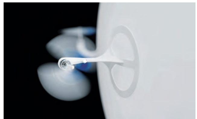
Vertical propellers: horizontal flying, accelerating and braking
