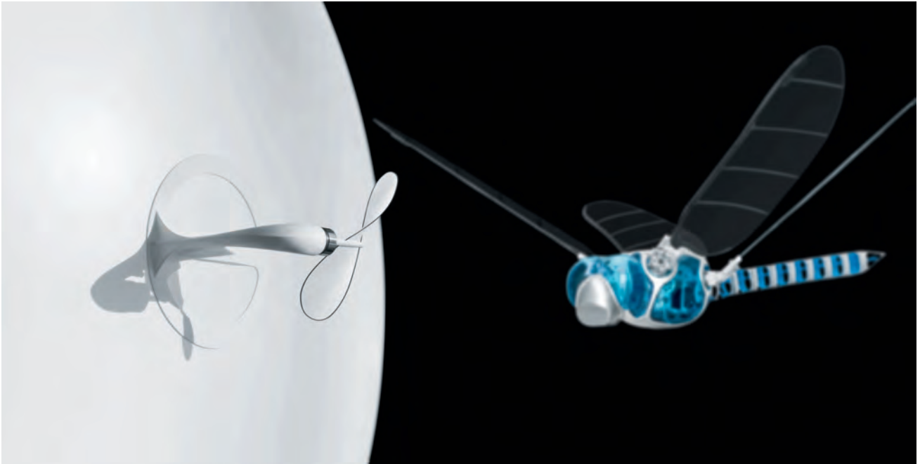
Pioneering role model: the BionicOpter wing principle transferred to the drive technology of the eMotionSpheres
